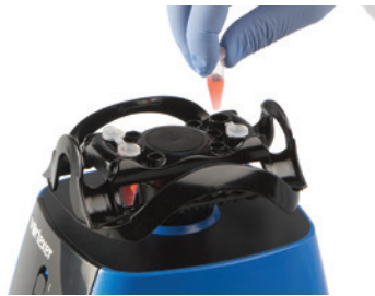
1.5/2 mL microfuge tubes x 4 (vertically mounted)
